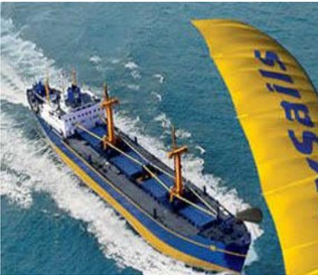
A company called SkySails is developing a range of giant kites for use by modern conventionally-powered freighters (see photo). SkySails kites, which can be as large as 320m<sup>2</sup>, are claimed to reduce a ship's annual average fuel costs by 10- 35%, depending on wind conditions. (ETA).
